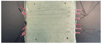
Piezoelectric (PZT) sensors encapsulation into veils will ensure their accurate placement in the structure and to protect them in service. NDI techniques will be used to validate the quality of the laminate.
