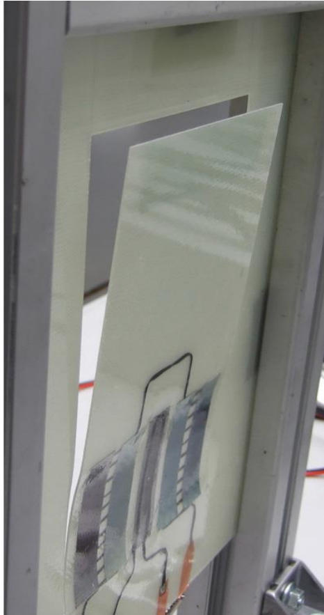
Glass fibre-reinforced sheet with embedded SMA actuators
