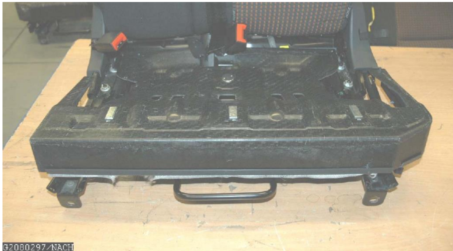
FRP seat pan after passed sled test
