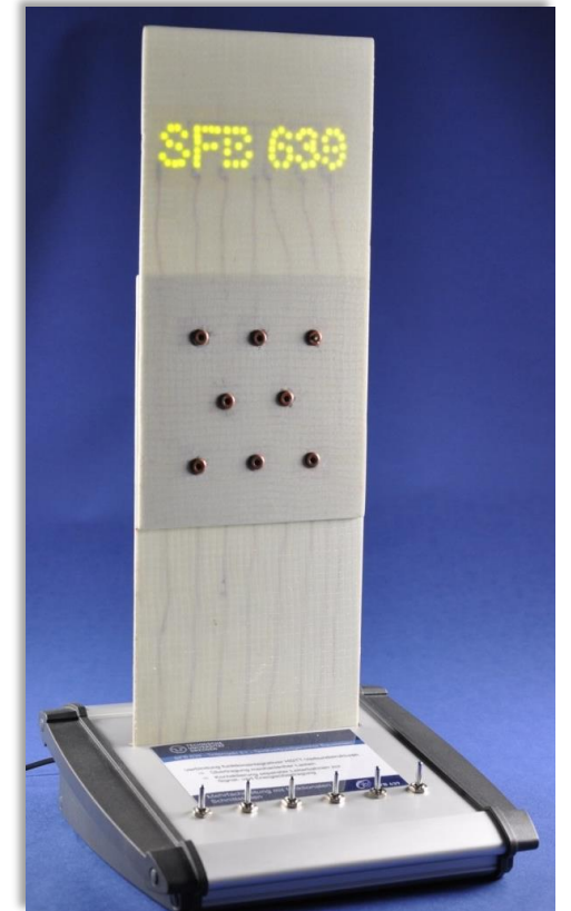
Integrated conductors and lighting elements in fibre-reinforced polymer
