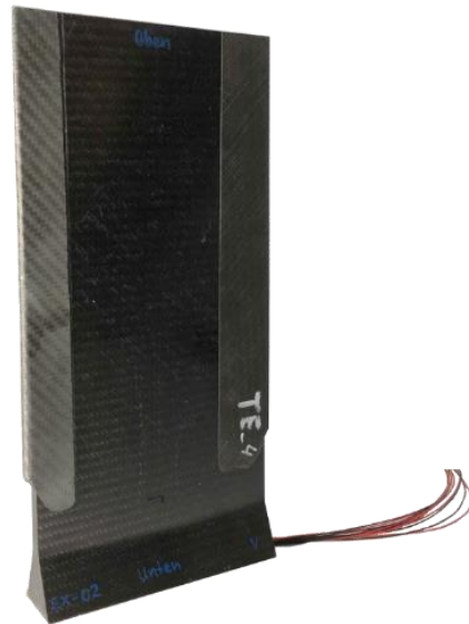
Blade with integrated sensor layer
